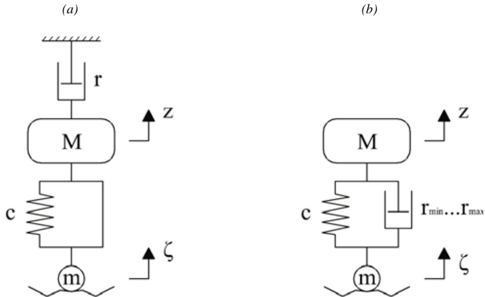
Fig. 1. Ideal sky-hook damping 1(a) and practical implementation of sky-hook damping 1(b)
