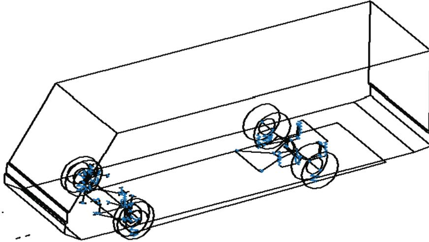
Fig. 2. Multidimensional model of the bus
