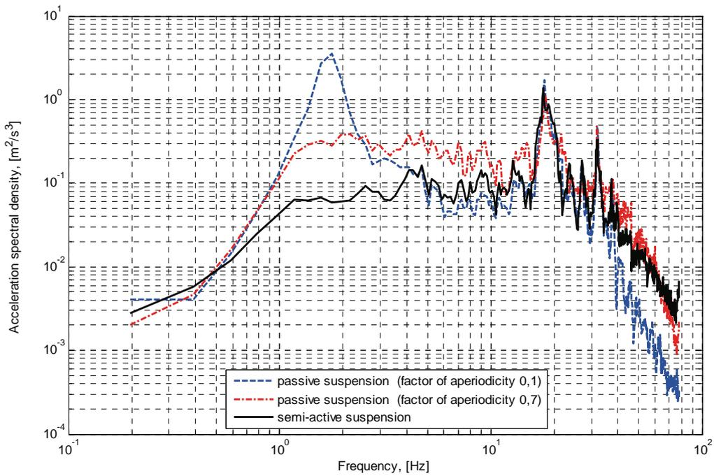
Fig. 4. Spectrums of vertical accelerations on a place of the driver
